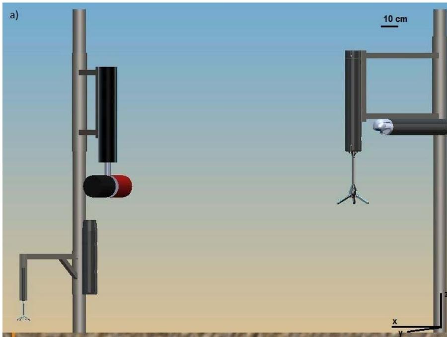
**Figure 6:** Instrumentation deployment method and relative locations in relation to sediment bed. Vectrino II (left) is 6 cm from bed, Vector (far right) is 0.8 m from bed, Aquadopp HR (horizontal, alignment on right) is 1 m from bed.
