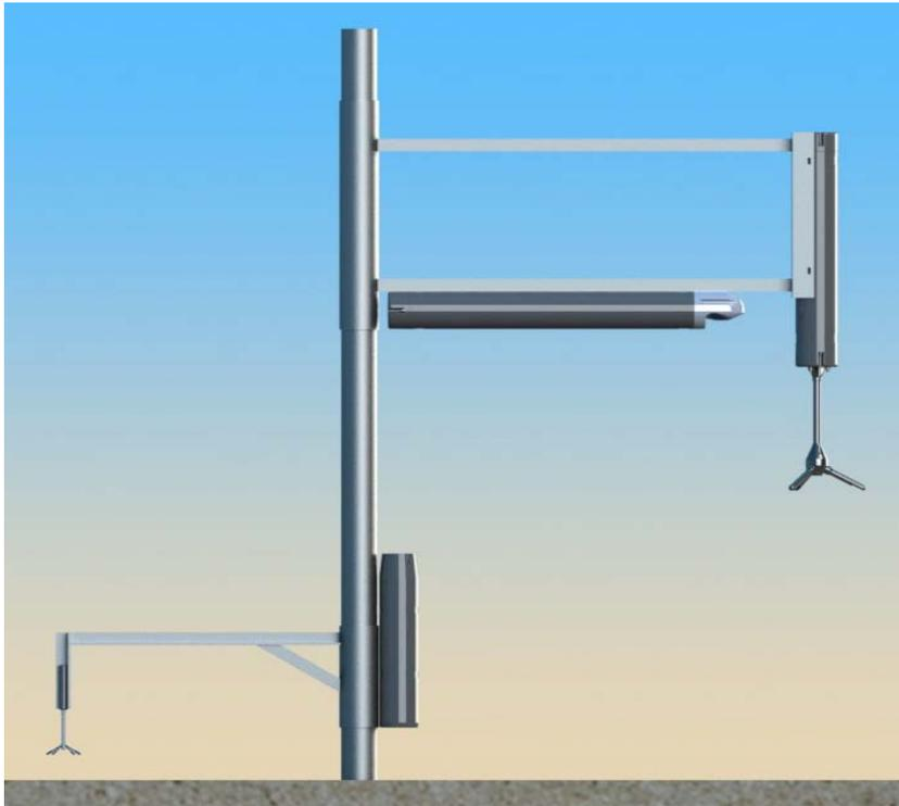
**Figure 4:** Instrumentation deployment method and relative locations in relation to sediment bed. Vectrino II (left) is 6 cm from bed, Vector (far right) is 0.8 m from bed, Aquadopp HR (horizontal, alignment to right) is 1 m from bed.
