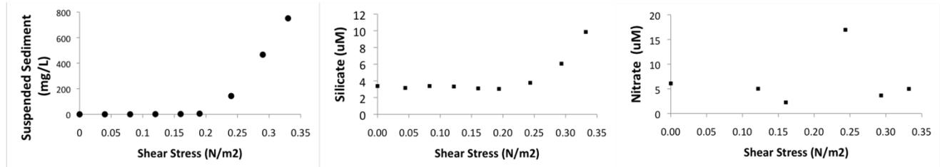
Figure 2. Erosion chamber experiment conducted at Thomas Point in Sept. 2010. The ammonium data has the same form as the silicate data but will not be available until an external calibration is complete. There was no phosphate release detected.
